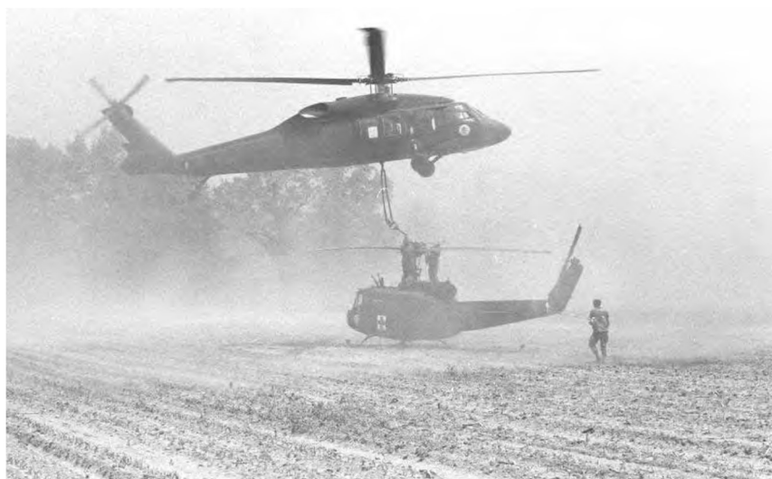
Swirls of dust from a dry cornfield in Michigan dramatically reduced visibility for Kentucky Army Guard pilots who were maneuvering their UH-60 Blackhawk to sling load a 6,800 pound disabled UH-1 Huey. Hooking cargo straps to the Huey's rotor hub are (l. to r.) SSG George Leffel and SSG Jim Whitaker. CW2 Jerry Watkins is on the ground holding the folded drogue parachute that trailed behind the load once it was in flight. (Photos by SFC Chuck Toler, KYARNG PAO) 1984.
