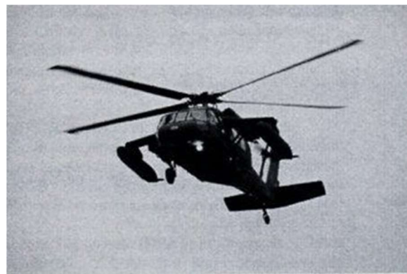
UH-60 Blackhawk with Extended Range Fuel System
